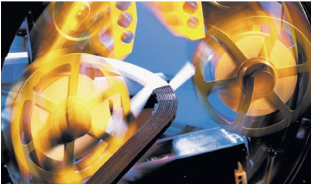
With high-speed taping machines Samicapor® und Samicatherm® tapes are precisely wrapped around the conductors.
